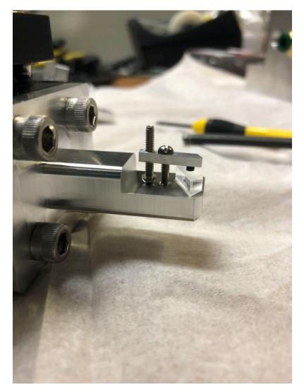
Figure A.5: BBO sitting in the custom mount, machined by Jim Kubasek. A small pocket was cut for the crystal to rest in, and the two-screw clamp holds it in place. The mount attaches directly to a stock Newport 9081 5-Axis aligner. A small piece of O-ring was placed between crystal and metal clamp to reduce mechanical stress on the crystal, which could induce unwanted birefringence.
