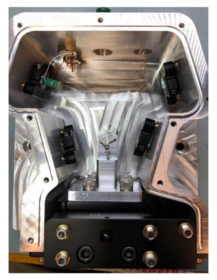
Figure A.7: Top view of the cavity, with the installed optics, crystal and crystal aligner, piezo and BNC connectors, and port for clean air displayed.
