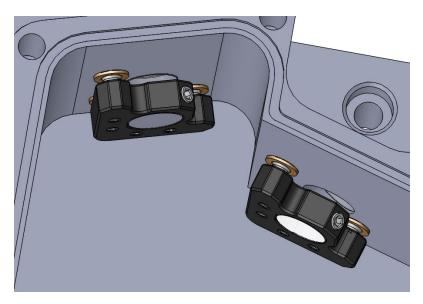
Figure A.3: SolidWorks rendering of the cavity's internal design. The mirror mounts were offset from the cavity wall in the model. The mirrors are offset from the wall in the real implementation so their angle can be changed. Also visible is the O-ring groove which helps provide an airtight seal for the cavity.
