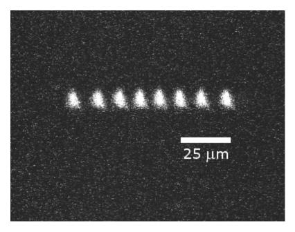
Figure 1.3: Beryllium ions trapped in the Paul Trap. The ions have been sufficiently cooled to the point where they form a Coulomb crystal, and the ions do not have sufficient energy to swap places with their neighbor in the lattice. Figure courtesy David Hanneke.
