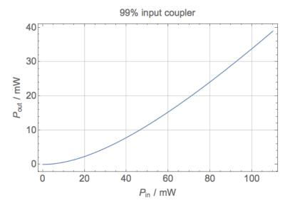
Figure 2.4: Second harmonic generation output power vs input power including Brewster losses for our cavity with optimal SHG and impedance matching with a 99% input coupler. At large input powers, the gain in the second harmonic output becomes linear as the loss of the fundamental becomes significant.
