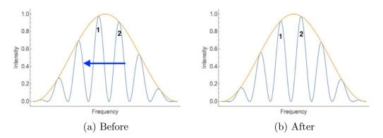
Figure 2.1: An external cavity diode laser, lasing at the frequency designated by (1) in 2.1a, switches to mode 2 in 2.1b as the external cavity mode (blue) drifts relative to the laser diode gain (orange). Once (1) surpasses (2) in amplitude, the laser starts lasing at the frequency of mode (2), causing a hop in the emitted frequency.
