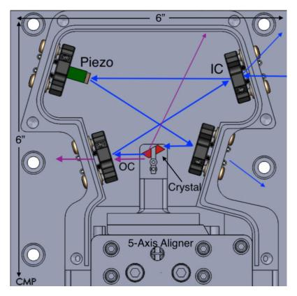
Figure 3.1: Solidworks rendering of the cavity design, including the path the 470 nm light takes (blue) and the path of the 235 nm light (violet).
