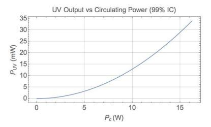
Figure 4.2: Plot of the output 235 nm power versus the circulating cavity power for a cavity on resonance and impedance matched with a 99% input coupler.
