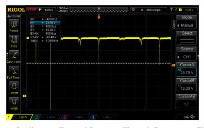
Figure 3.4: Oscilloscope Trace of Scanning Through Resonance. The large, narrow dips in power correspond to the piezo sweeping through resonance of the Gaussian mode. The smaller dips are higher order modes becoming resonant in the cavity. This figure displays close to the maximum amount of input light which was coupled in (45%).
