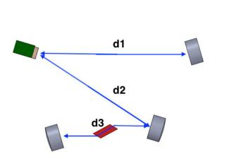
Figure 2.3: Symmetric bowtie cavity and illustrations of lengths used in calculating cavity parameters.  $d_3$  includes the length of the crystal, adjusted for the index of refraction.
