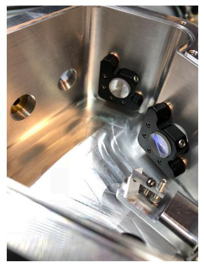
Figure A.6: Internal view of the cavity with the mirror mounts with mirrors installed. Also visible is the hole for the 235 nm light which reflects off the Brewster's cut of the crystal to exit the cavity. The hole is angled with respect to the cavity wall so allow the Brewster reflection to egress. It is also threaded for optics retaining rings to add a window.
