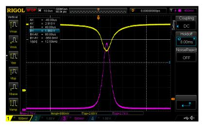
Figure 3.5: Oscilloscope Trace of Blue and UV Buildup. The increase in UV power out (purple trace) is correlated with the buildup in blue light in the cavity (yellow trace), which appears here as the loss of reflected light off the cavity.
