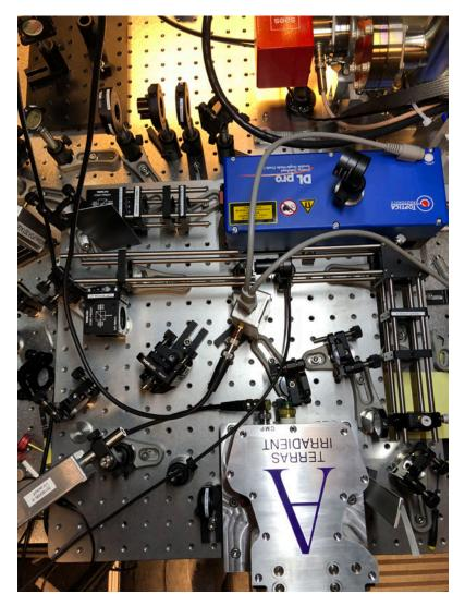
Figure A.9: Cavity along with the other pieces of the laser system, including the ECDL laser head, input optics, and photodetector for measuring the reflection off the input coupler, all mounted to the same optical breadboard. The breadboard will support additional components for locking and fibers optic cables to feed to the frequency stabilization system.
