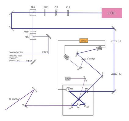
Figure 3.2: Beryllium Photoionization Laser System. Blue light from the ECDL is coupled into the power enhancement cavity to increase the amount of UV light produced by second harmonic generation. The elements which make up the feedback control system are detailed in Section 4.3.
