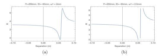
Figure 4.1: Calculations of the required lens separation between a 250 mm lens and -50 mm lens to bring a beam to a focus, varying the distance between the lenses. The left is for an input beam with a 2 mm spot size (approximate input beam size), while the right is for a slightly larger beam at 2.5 mm. For the slightly larger size, there is no configuration where the beam comes to a focus (stable solution for where  $R = \infty$ .)
