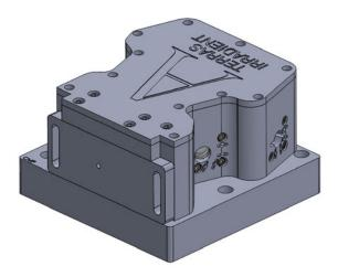
Figure A.1: SolidWorks rendering of the cavity. The thickness of the base was adjusted so that the center of the mirrors in the cavity are at the same height of the beam emitted from the aperture of the ECDL. The lid helps seal the cavity from contaminants, which may adhere to the optics. The base is 6 inches wide by 6 inches tall.
