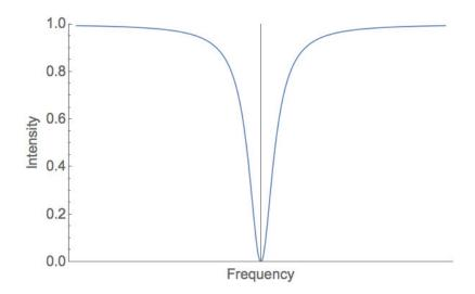
Figure 4.3: Plot of the reflected power versus frequency for a cavity close to resonance.
