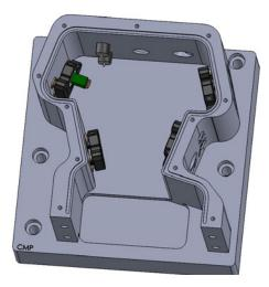
Figure A.2: The crystal aligner has been removed from the SolidWorks model, exposing the pocket in the cavity floor to allow the crystal aligner to move through its entire range of motion.
