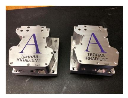
Figure A.4: The pair of cavities machined by Jim Kubasek in the Amherst Machine Shop. The lids have holes for screws to fasten the lid and main body together. There are also holes to access the crystal aligner adjustment knobs without taking off the lid. Minus the lid, the entire cavity was machined from a single block of aluminum.
