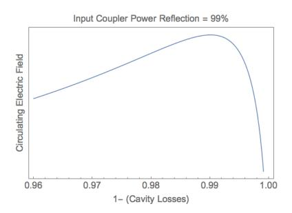
Figure 2.5: Circulating electric field versus choices for the coefficient of reflection for a 99% input coupler. Note the maximum occurs when the round trip cavity losses equal the transmission of the input coupler.
