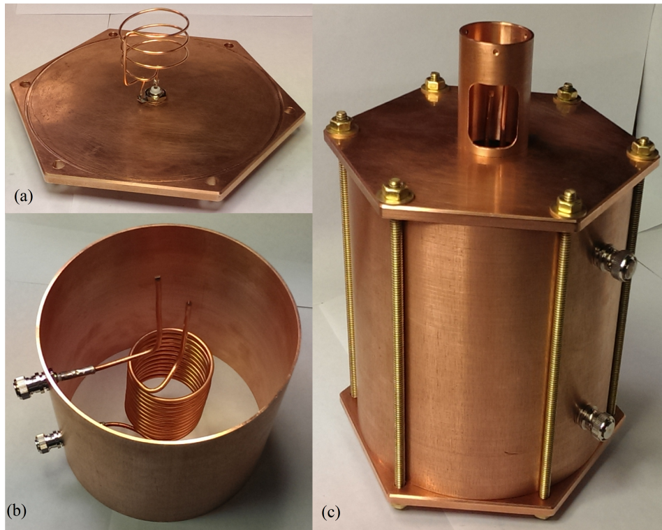
Figure 4.1: Picture of the fully constructed resonator. (a) Base plate of the resonator with the antenna coil. (b) Inside the shield showing the main coil and the ground rod. (c) The resonator assembled and ready to be connected to the ion trap via a vacuum feedthrough.
