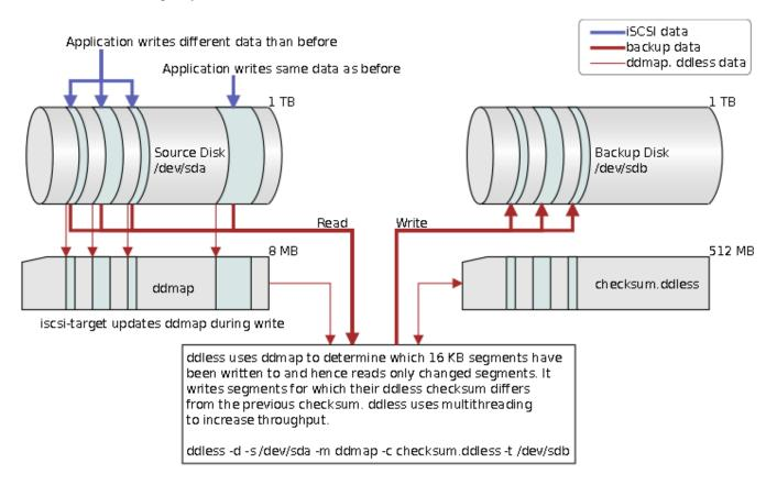
Figure 3: Using ddless and ddmap, read changed data and write changed data
