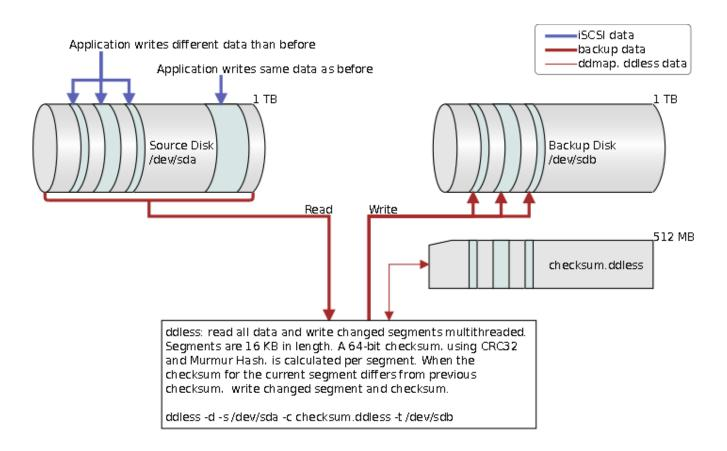
Figure 20: Using ddless, read all data and write changed data
