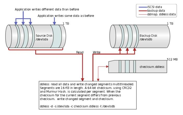
Figure 2: Using ddless, read all data and write changed data
