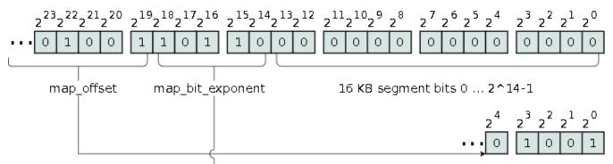
The map\_offset value is derived from bits 19 through 63. The bits are shifted to the right 19 times. The resulting range is 0 ... 2^45-1 or 32 TB. The above map\_offset value is 9.
