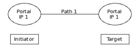
Figure 14: Single path with 1 network portal at the initiator and 1 network portal at the target
