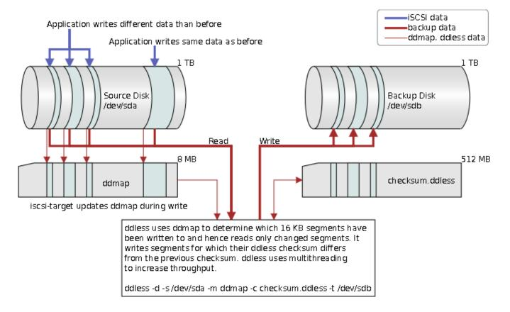
Figure 21: Using ddless and ddmap, read changed data and write changed data
