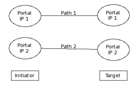
Figure 17: Multipathing with 2 network portals at the initiator and the target using the iscsi-portal
