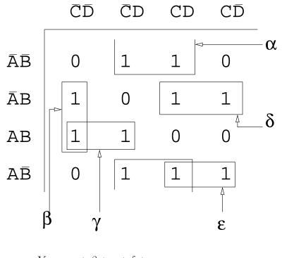
$\begin{array}{rll} Y = & \alpha + \beta + \gamma + \delta + \epsilon \\ = & \bar{B}D + B\bar{C}\bar{D} + AB\bar{C} + \bar{A}BC + A\bar{B}C \end{array}$
